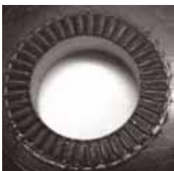
Painted surface after use of NORD-LOCK with standard diameter
