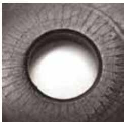
Painted surface after use of NORD-LOCK with enlarged outer diameter
